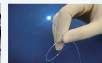
iber scope using image fiber
