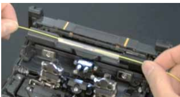
Fig. 4. Conventional splice sleeve positioning groove.
