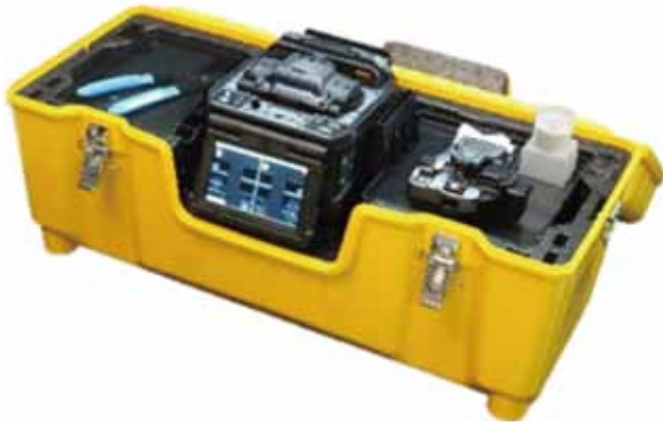
Fig. 7. Opened carrying case (with work tray inside enabling splicing operation).
