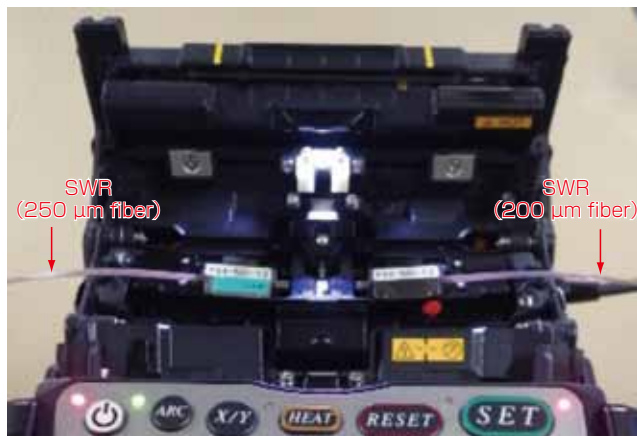
図3 250μm SWRと200μm SWRの融着接続 Fig. 3. Fusion Splicing of Spider Web Ribbon (200 μm Fibers and 250 μm Fibers).
