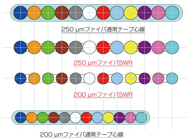
図2 200 μmF-SWRのファイバピッチ設計 Fig. 2. Design concept of SWR using 200 μm fibers.
