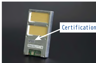
Pre-certified 60 GHz millimeter-wave communication module
