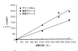
図7 塩水噴霧試験後のACSRの孔食深さ Pitting depths of ACSR after salt spray test
