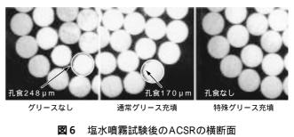
Cross sections of ACSR after salt spray test
