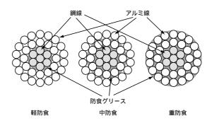
図1 防食電線の構造例 Examples of corrosion-resistant conductor structure
