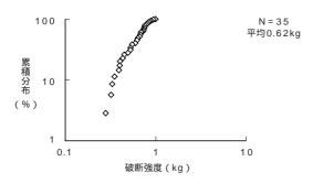
図8 融着部の累積破断確率 Cumulative failure probability of splice strength
