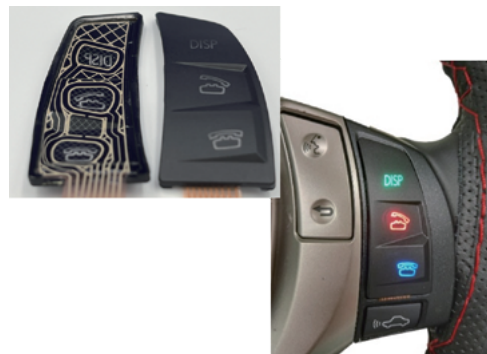
■ Figure 2 : Electrostatic capacitance type 3D switch (Base Material: polycarbonate)
