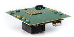
28 GHz mmWave phased array antenna module (PAAM)
