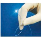
Ultra-thin fiberscope using image fibers
