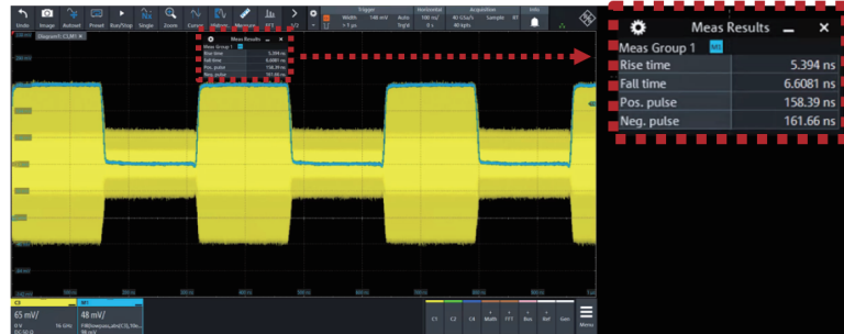
Fig. 15. Beam switching time of 256 elements PAAM.
