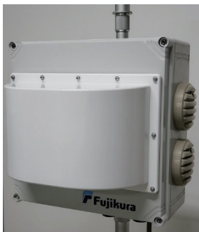
Fig. 5. 60 GHz wide-band communication module mounted on chassis.
