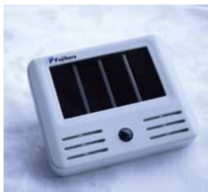
Fig. 1. Wireless temperature/humidity/motion sensor powered by a 4-series DSC module.
