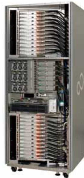
Fig. 12. Rack of Fujitsu's super computer "K" equipped with cold plate unit.
