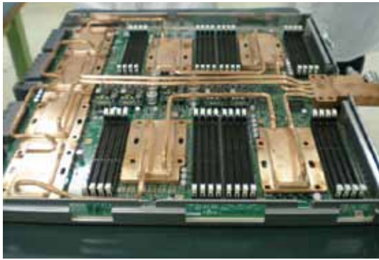
Fig. 11. Photo of cold plate module assembled on system board of super computer.
