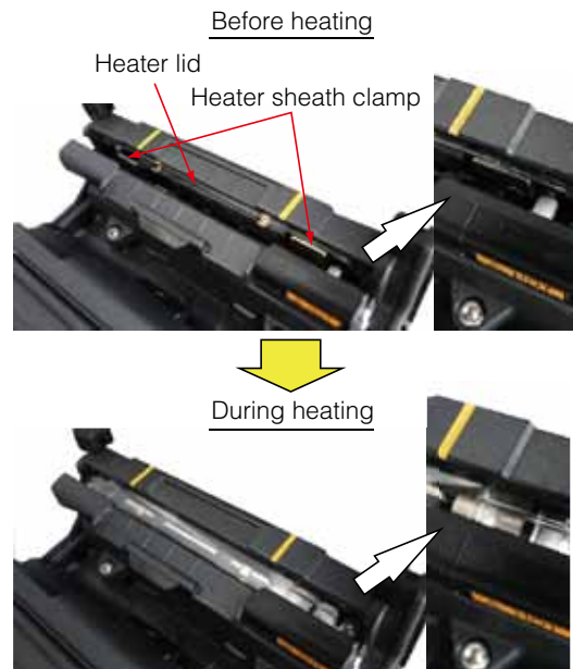
Fig. 6. Automatic open-close function of tube heater.
