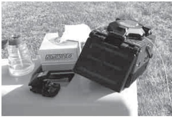
Fig.3. Splicing on unstable surface.
