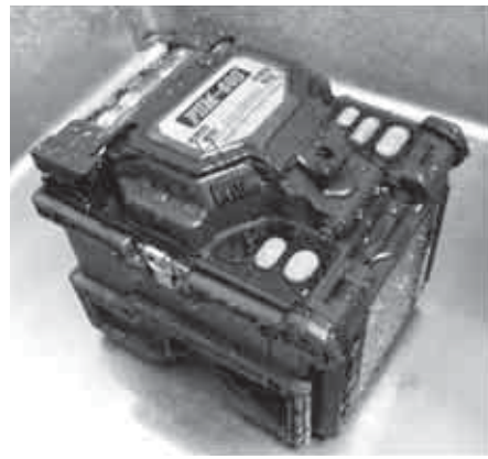
Fig.15. Appearance after rain test.
