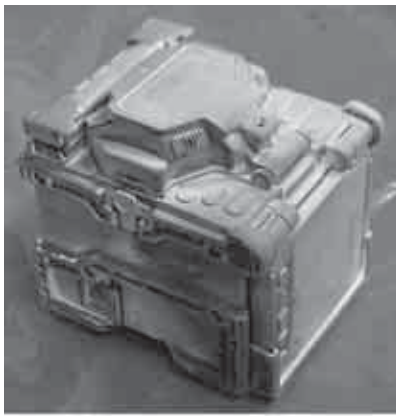
Fig.13. Appearance after dust test.
