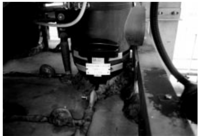
図4 光磁界センサ外観 Appearance of optical magnetic-field sensor
