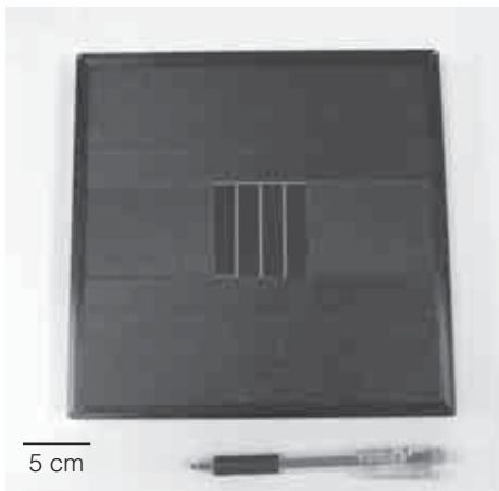
Fig. 9. An appearance of the robust DSC with novel package for the endurance tests.
