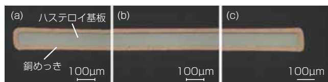
図 5 銅めっき線材の断面写真 (a)(c) 幅方向エッジ部 (b) 幅方向中央部 Fig. 5. Cross-sectional photographs of copper plated wire. (a)(c) Both edges across the width direction. (b) Center part across the width direction
