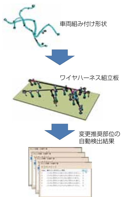
図12 3次元CADを活用した製造設計の効率化 Fig. 12 Efficient method for wire harness manufacturing design by use of 3D CAD.
