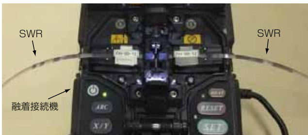
図2 12心SWRの融着接続 Fig. 2. Fusion splicing of SWR.
