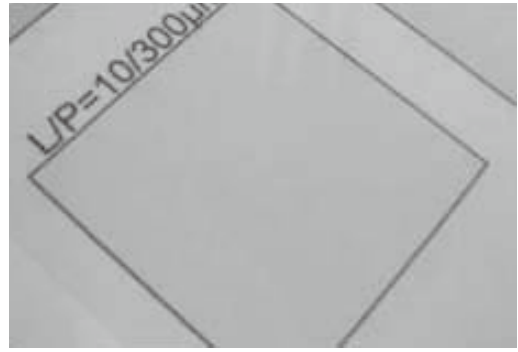
図8 透明電極用微細銀メッシュパターン外観 Fig. 8. Appearance of fine Ag mesh traces for transparent electrode.
