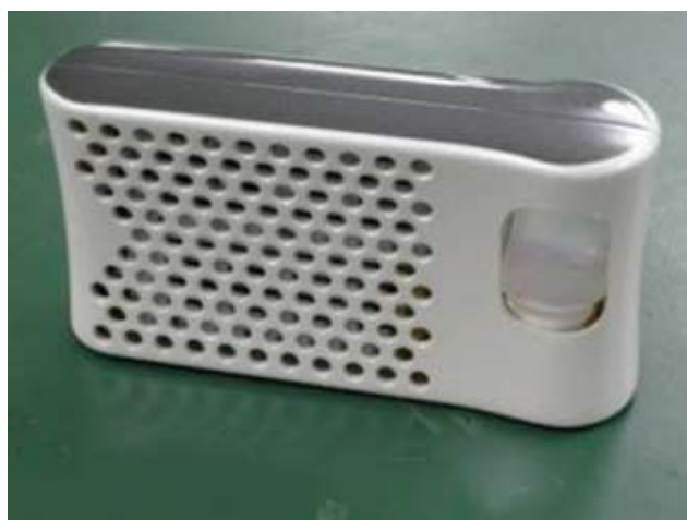
図6 小型携帯型電子機器用DMFC Fig. 6. DMFC for small portable electronic device.
