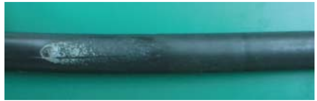
図6 難燃試験後のシース状況(UL-1581 VW-1) Fig. 6. Picture of sheas after flame test (UL-1581 VW-1).
