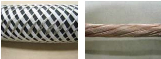
図5 低温捻回試験後の遮へい層, 導体の状況 Fig. 5. Picture of shield wire and conductor after low-temperature twisting test.
