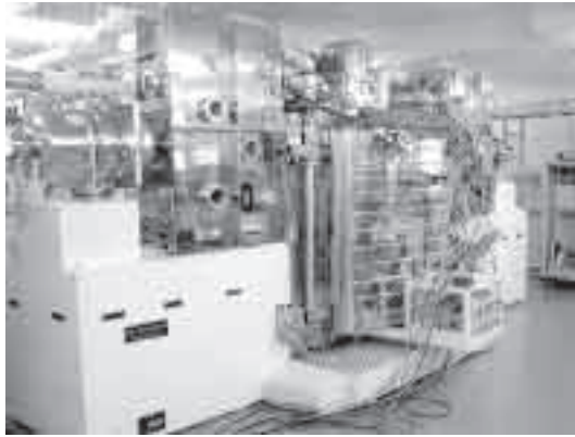
図5 大型IBAD装置の外観と模式図 Fig. 5. Photograph and schematic of large-scale IBAD system.
