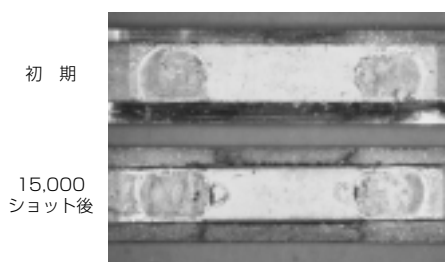
図6 端子溶接部外観 Appearance of welding point
