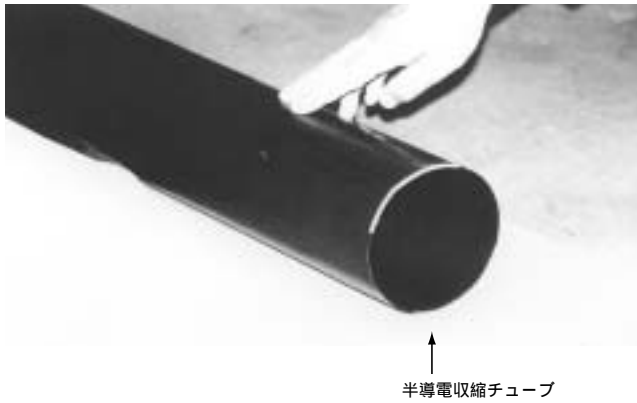
図16 曲面抵抗体の測定用サンプル A sample of curved surface resistor for measuring
