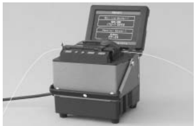
図5 操作方向の変更機能 Change of operating direction
