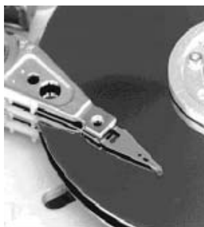
図1 HDDのサスペンションの外観 Appearances of suspension in hard disk drive
