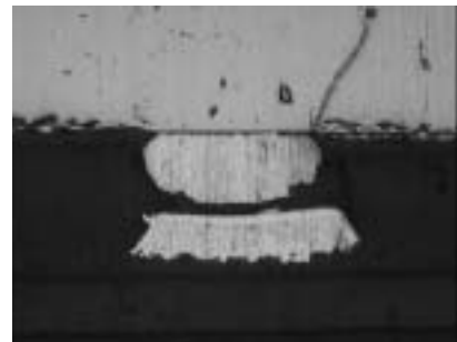
図6 アンダーフィル硬化時破断例 Cross section view of rupture after underfill resin hardening
