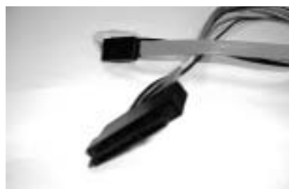
図2 Serial ATA Overlook of Serial ATA
