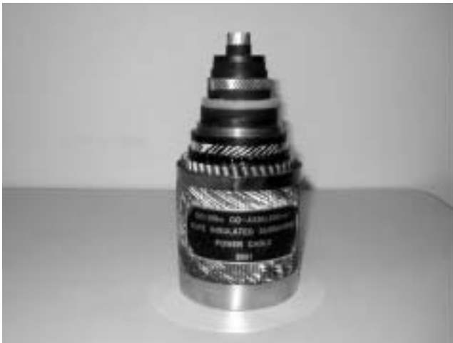
図1 直流120kV同軸CV海底ケーブルの外観 External view of DC120kV coaxial type extruded insulation cable
