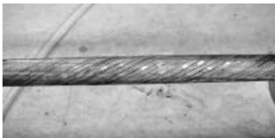
図5 帰路導体溶接部 Welding portion of return conductor
