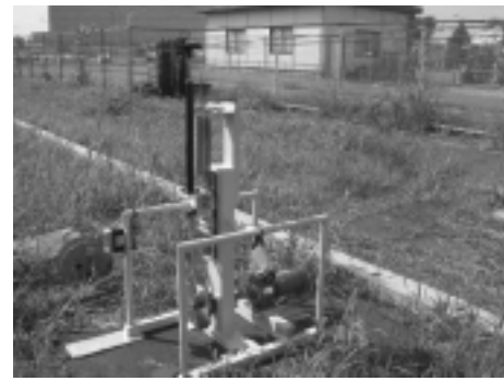
図 10 加振機 Photograph of dancing test equipment
