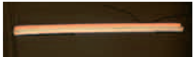
図8 Cu安定化層複合線材 Fig. 8. Cross section view of Y-123 with Cu stabilizer.
