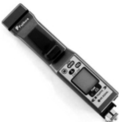
図2 新型心線対照器の外観 Fig. 2. Appearance of new optical fiber identifier.
