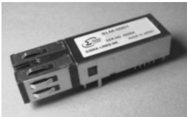
図4 新開発光トランシーバ外観 Fig. 4. Outer shape of proposed optical transceiver.
