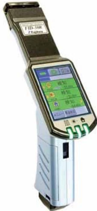
図7 ONU検知機能付き心線対照器 外観 Fig. 7. Appearance of new optical identifier with ONU detecting function.
