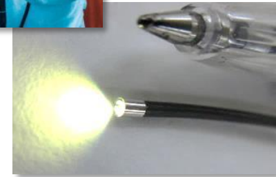
E.g.: Ultra-thin \phi 1.3-mm CMOS endoscope
