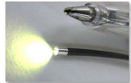
Example: CMOS endoscopy camera with extremely narrow diameter of \phi 1.3\text{mm}
