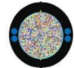
1,728 core Wrapping Tube Cable® (WTC®)
