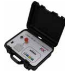
LISSA-100 live sheath and shield resistance measuring device
