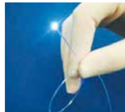
Fiberscope using image fibers
