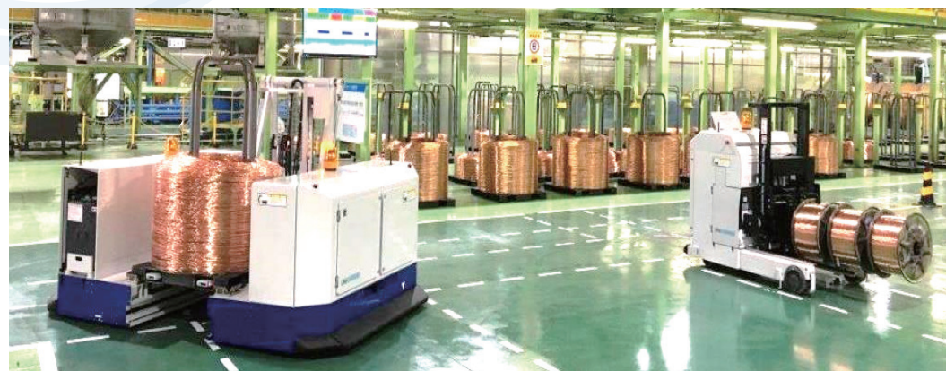
● Cable material automatic carrying system
