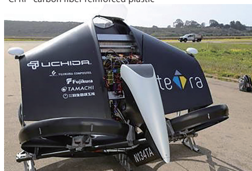
● Flying device with vertical take-off and landing abilities, tetra 3
