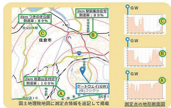
● Wireless environment field test in Chiba City, Chiba Prefecture
