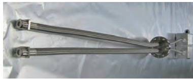
● Outlook of light guide for ultrahigh vacuum environment ● Edge on vacuum side (eight optical fibers in line)
